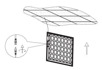
2. Connect the power line, then put LED panel on the ceiling screens.
