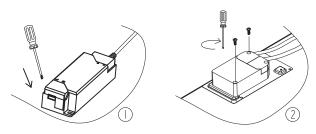
1. Connect the power input wire, then fixed power supply.
