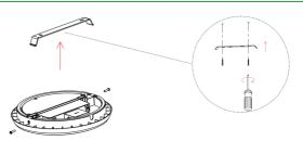
Remove screw, take out bracket and fix it with screw into the ceiling.
