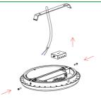
Open junction box, wire "l" "N" to terminal block and mount ceiling light into the right place.
