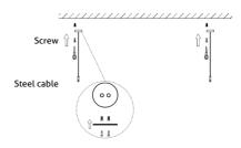
Screw the clip on the ceiling tightly.
