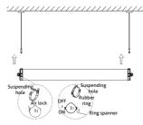
Hung the fixture under the steel cable and secure the fixture by steel cable
